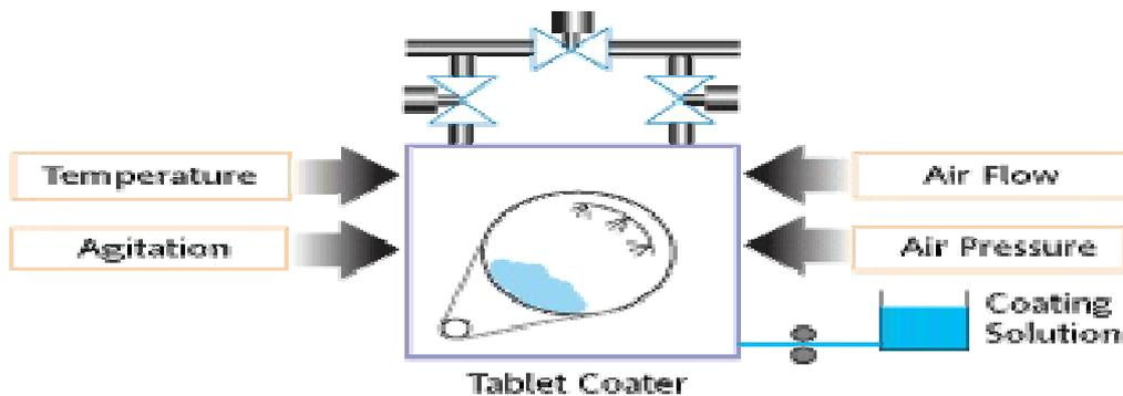
The liquid spray coating is then dried onto the tablets by heated air drawn through the tablet bed from an inlet fan. The air flow is regulated for temperature and volume to provide controlled drying and extracting rates, and at the same time, maintaining the drum pressure slightly negative relative to the room in order to provide a completely isolated process atmosphere for the operator.
